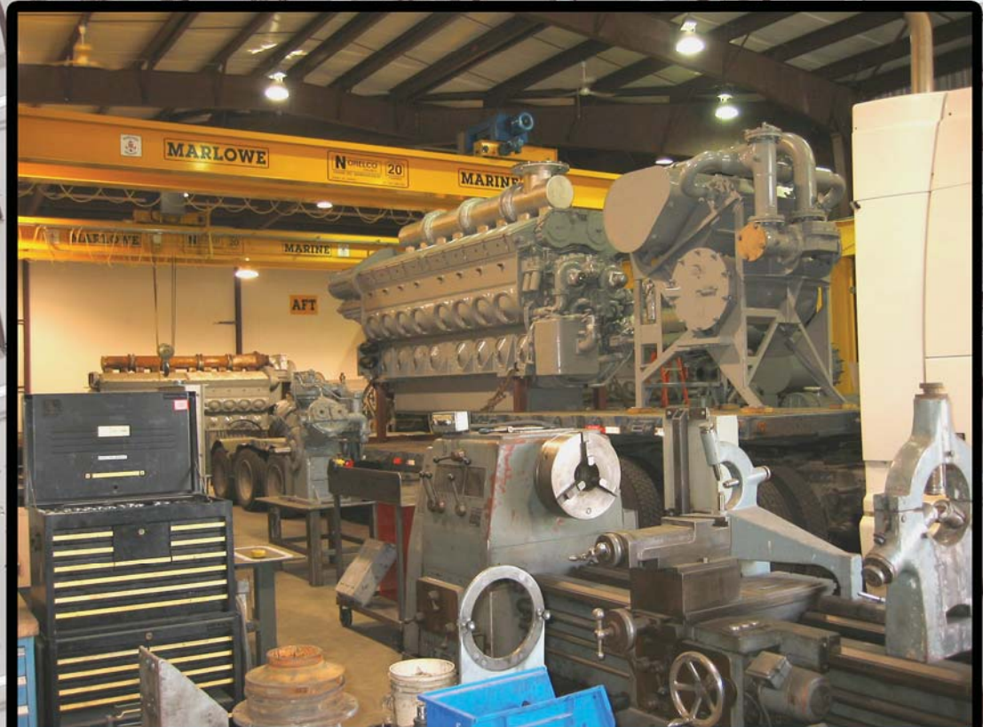
CONVERSION OF 16-645E3 TURBO TO MARINE 16-645E6 ROOTS
