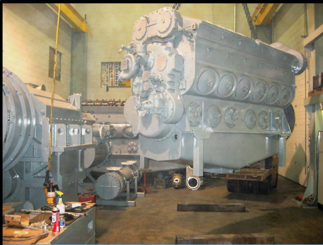
CONVERSION OF 12-567C TO MARINE RIGHT HAND ROTATION 12-645C2
